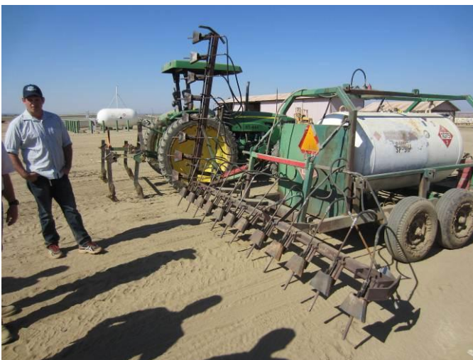
One of Grimmway's propane burners used as a weed killer in both conventional and organic carrot fields.
